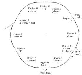
Figure 1: Layout of the High Energy Ring
