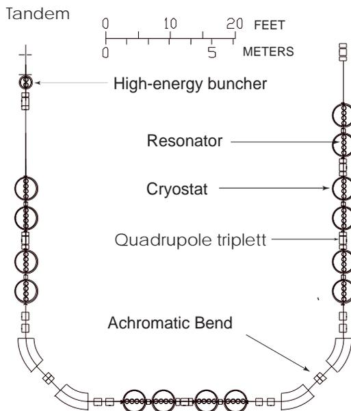
**Figure 2** The linac has 14 cryostats, each cooling 4 niobium superconducting  $1/4\lambda$  resonators. The configuration depicted uses quadrupole triplets for transverse focusing. Achromatic bends are used to wrap the linac back upon itself.
