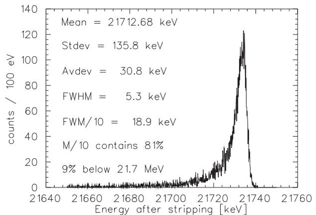
**Figure 3** Beam energy spread from stripping  $^{175}\text{Lu}$  to  $15+$  in an equilibrium thickness  $^{12}\text{C}$  foil, in the tandem terminal. This translates into time spreading, and is a major component of the time spreading in the tandem beam  $\sim 1 \text{ ns}$ .
