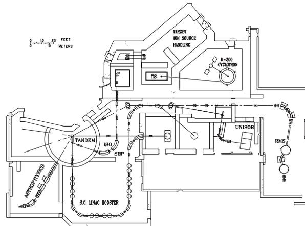
**Figure 1** Floor plan depicting the conversion of the HRIBF into the National ISOL Facility. The main changes are a new driver accelerator, a modified target ion source platform, and the addition of a superconducting linac to boost the tandem beam.
