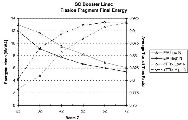
**Figure 4** Final beam energy of useable fission fragments as a function of Z. Results for both the high and low mass useable fission fragments are shown. Also shown are the corresponding average transit time factors. Optimized for high masses, the SC linac is still efficient over the fission fragment mass range.
