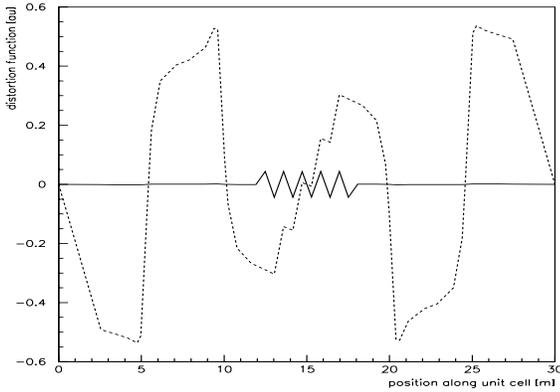
Figure 1: Distortion function  $B_1$  for the matched (line) and unmatched (dotted line) case along one BESSY II cell.
