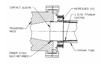
Figure 2 - Ceramic Tube End Joint Design
