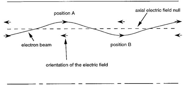
Figure 1. Rippled beam interaction, showing single electron synchronism.
