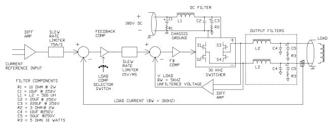
Figure 1, Regulator Configuration
