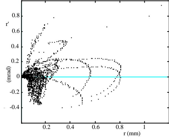
Figure 2b: Particle distribution in transverse trace space (r,r') at the location of minimum emittance
