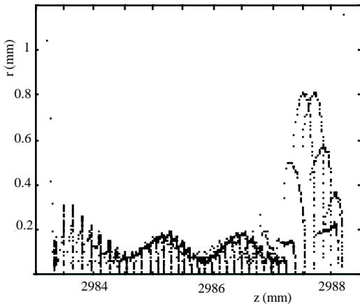
Figure 2a: Particle distribution in the configuration space (r,z) at the location of minimum emittance
