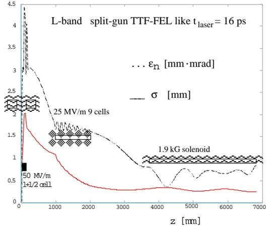
Figure 3: Envelope and emittance behavior of a beam matched from the IE to Brillouin flow with local correction of bifurcated tails
