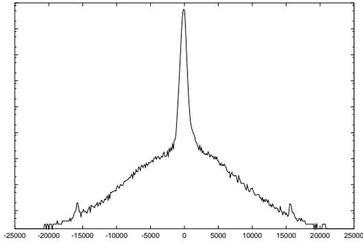
Figure 1: The RF generator spectrum about  $\omega_{RF} = 499.765$  MHz.
