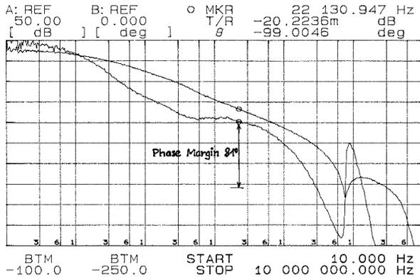
Figure 3 : Open-loop transfer function
