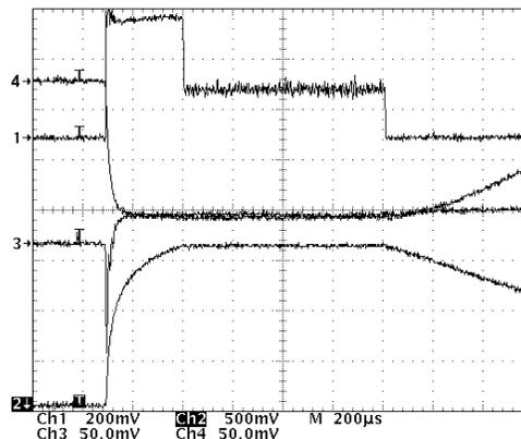
Figure 7 : Without beam, incident power (trace 1), field amplitude (2), field phase (3), phase reference (4)
