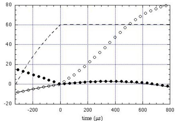
Figure 1 : Cavity phase (in degrees) a) without beam  $\Delta f = 80 \text{ Hz}$  (solid line), b) with beam  $\Delta f = 80 \text{ Hz}$  (empty circles), c) with beam  $\Delta f = -120 \text{ Hz}$  (solid circles)
