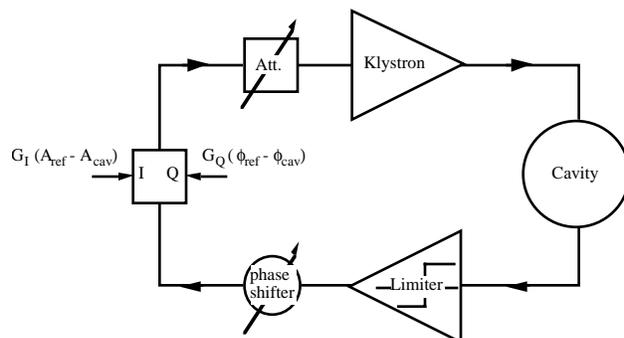
Figure 2 : Schematic drawing of the control loops.
