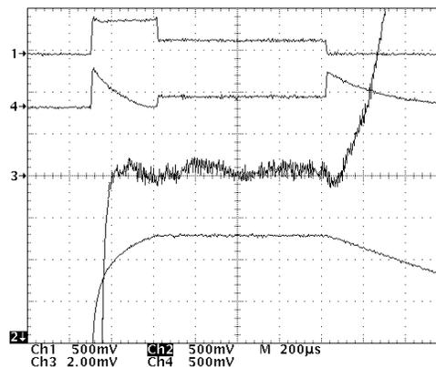
Figure 8 : Without beam, incident power (trace 1), field amplitude (2), field phase (3), reflected power (4)
