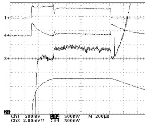
Figure 9 : With beam, incident power (trace 1), field amplitude (2), field phase (3), reflected power (4)
