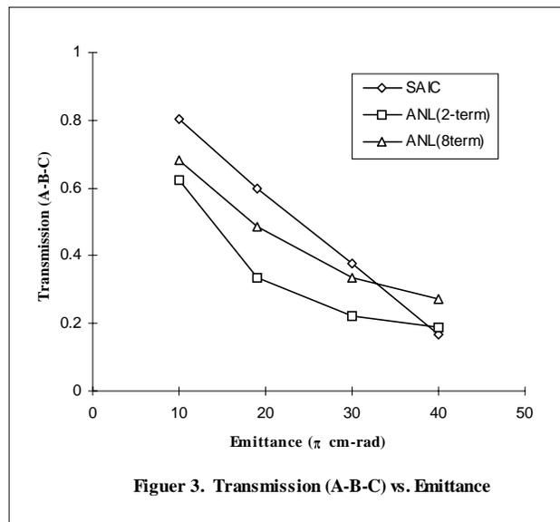
Figure 3. Transmission (A-B-C) vs. Emittance
