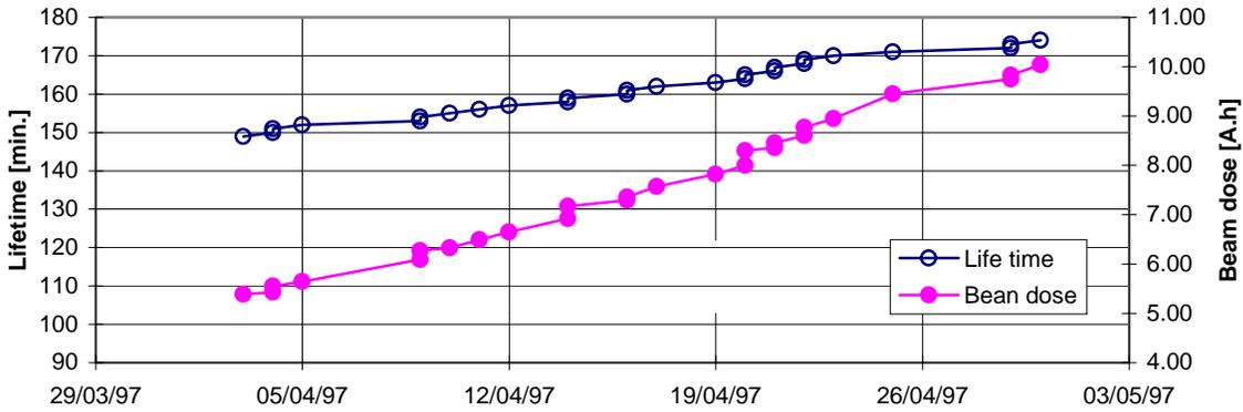
Figure 1: Beam lifetime at 40 mA and the integrated beam dose
