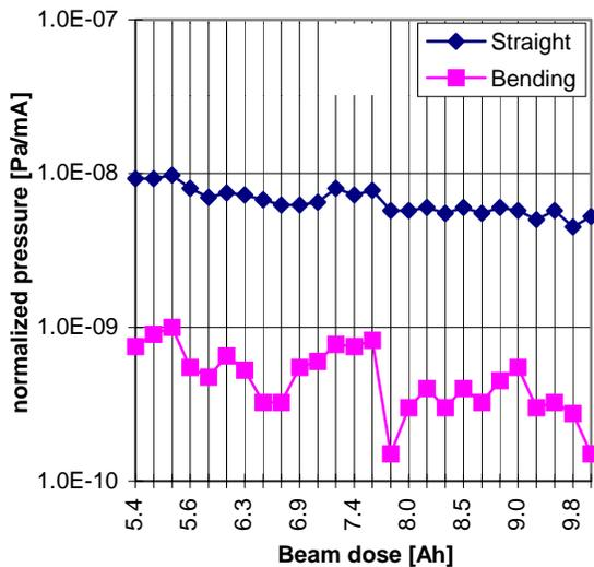
Figure 2: Normalized pressure at bending and straight chambers
