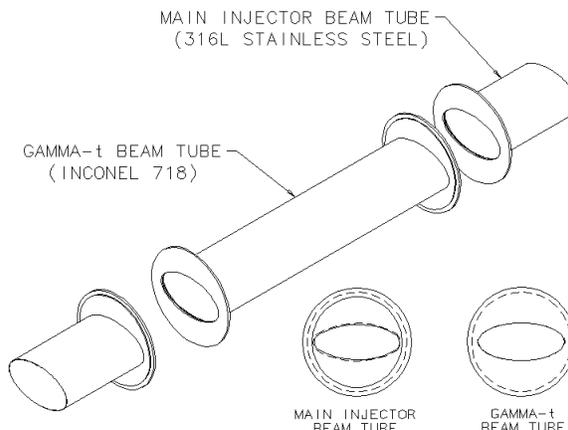
Figure 6: Isometric drawing of FNAL Main Injector  $\gamma_t$ -jump system beamtube design.
