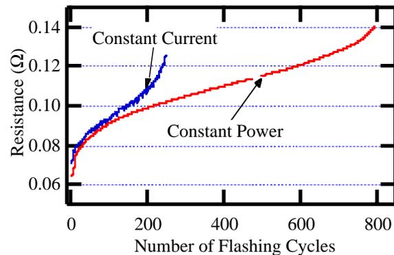
Figure 2. Resistance of Ti filaments during Ti flashing
