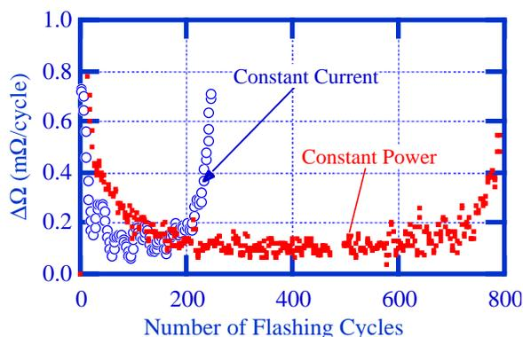
Figure 3. Resistance change rate of Ti filaments, as derived from the results shown in Figure 2.
