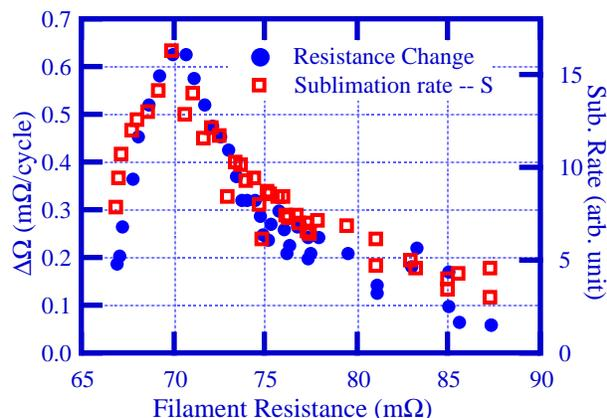
Figure 4. Resistance change rate and relative sublimation rate as a function of Ti filament resistance.
