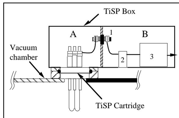
Figure 1. Schematic of CESR interaction region TiSP box. (1)Capacitance feedthroughs; (2)DC contacts (3)LC / RC filter networks
