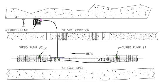
Figure 1: APS storage ring with ancillary pumping system.
