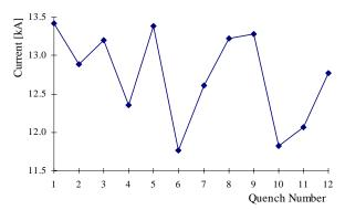
Figure 3: Quench pattern after the cycling experiment
