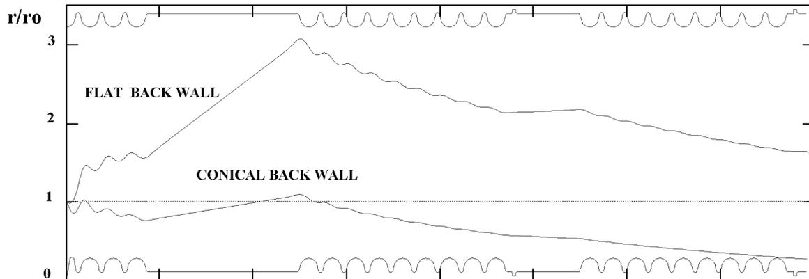
**Figure 2.** Beam radius in the accelerator: with flat back wall and with conical back wall.
