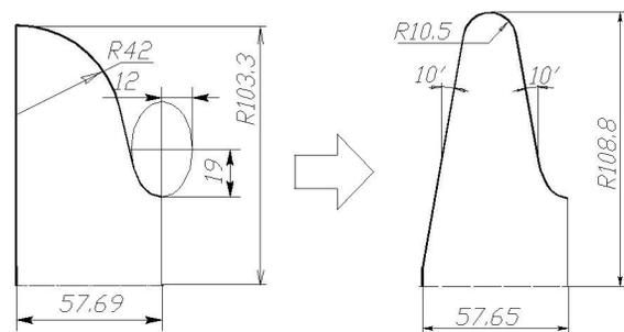
Figure 1. Accelerator RF-gun first cells.
