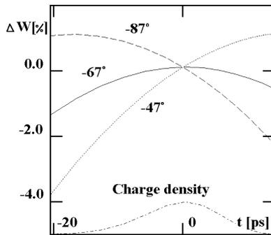
**Figure 3.** Beam energy distribution at the accelerator exit
