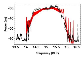
Fig 1: Power spectrum radiated to the downstream HOM coupler: experimental values are shown dashed and those calculated from circuit theory are indicated by the solid curve.
