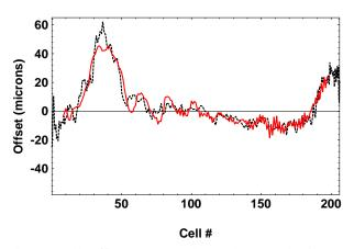
Fig 7: Cell offsets computed by the pseudo inverse method(solid curve) compared to those computed by remapping as in Figs. 5 and 6 (dashed curve).
