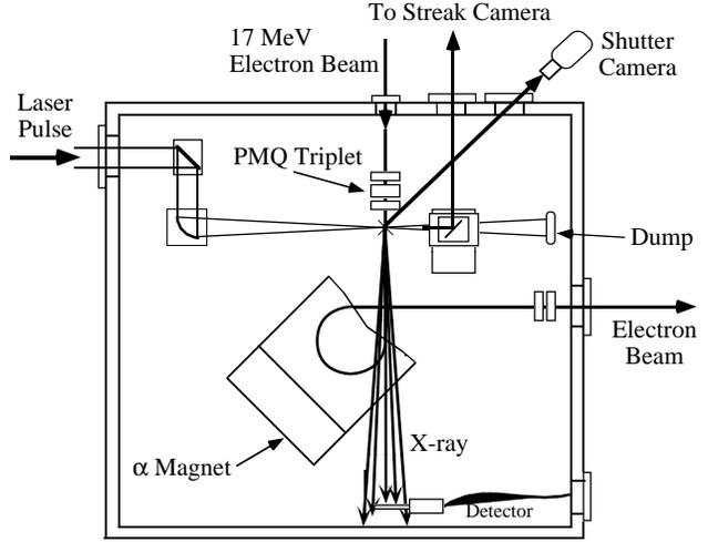
Figure 1: The experimental setup for  $90^\circ$  Thomson scattering.
