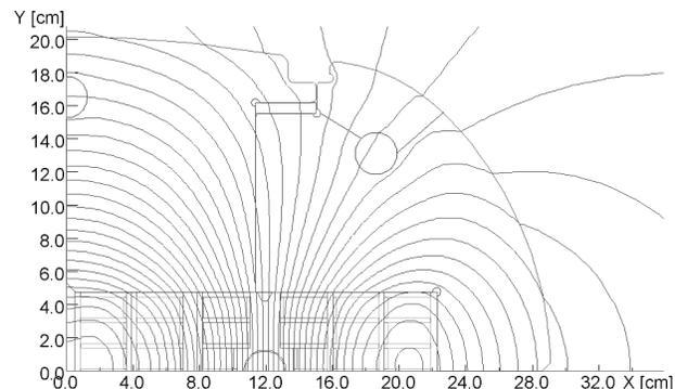
Fig.1. 2D view of the magnet with the field lines.
