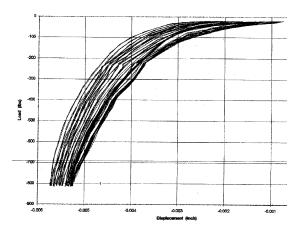
Figure 4. Laminar spring stress/strain: 10,000 cycles.
