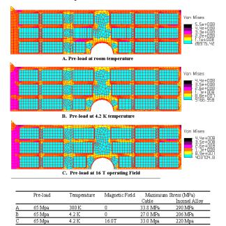
Figure 6. Finite-element calculations of the stress and strain distributions in the 16 Tesla dual dipole.
