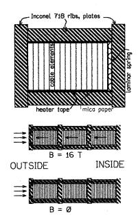
Figure 2. Detail of stress management in a coil block.
