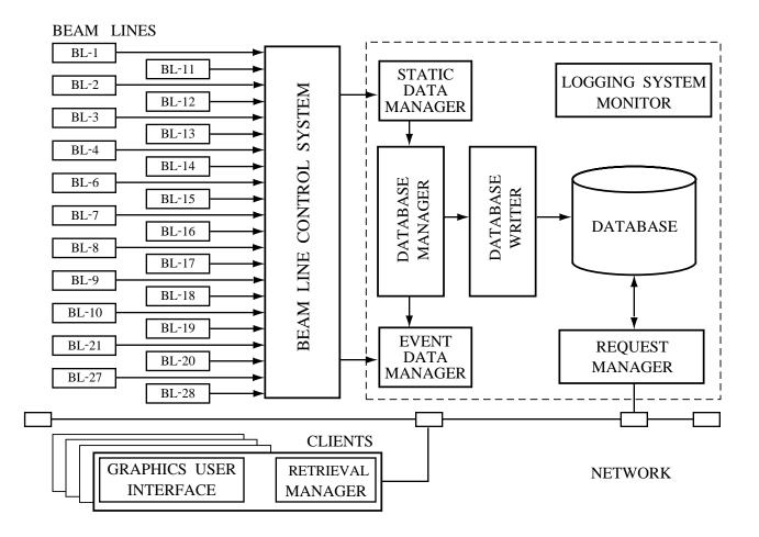
Figure: 1 Block diagram of the Operation Logging System for Synchrotron Radiation Beam Lines
