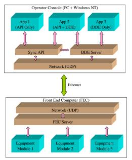
Figure 2: Data Flow from Console to FEC
