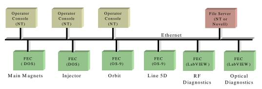
Figure 1: Layout of the upgraded SRS Control System
