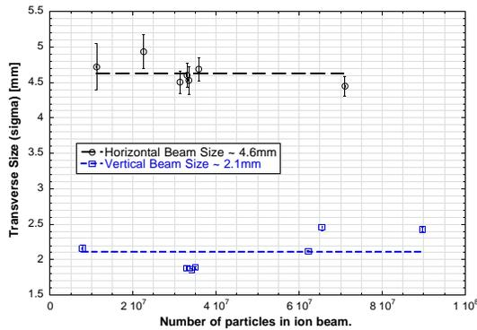
Figure 4: Horizontal and vertical beam sizes measured for uncooled beams having various particles numbers (measured bunch lengths (FWHM) =  $1.00\text{m} \pm 0.05\text{m}$ ). The longitudinal velocity spread is of order 600 m/s for all measurements.
