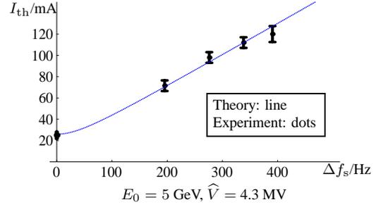
Figure 7:  $I_{th}(\Delta f_s)$ , theory and experiment.
