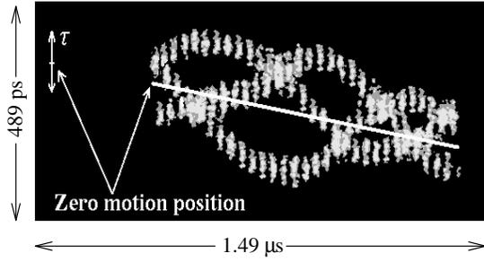
Figure 4: Instability in a 1/3 filling.
