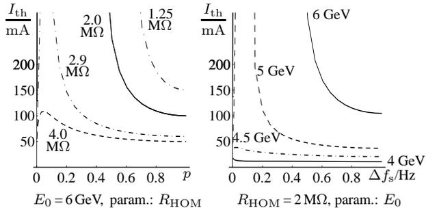
Figure 6:  $I_{th}(p)$  from eq. (9),  $f_{HOM} = 500$  MHz.
