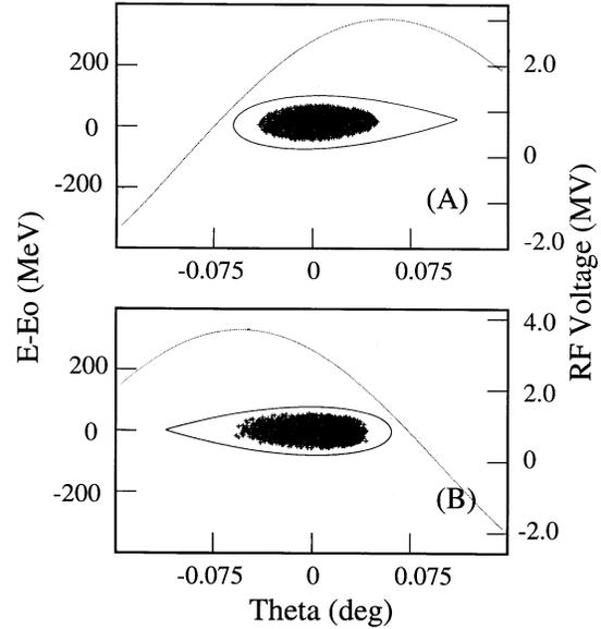
Figure 2: Phase space distribution (i.e.,  $\Delta E$  vs  $\theta = \Delta\phi$ ) of 0.25 eV-sec proton bunch in an accelerating rf bucket in the Main Injector with 53 MHz rf system. The closed contours represent the buckets for the case at 20 msec (A) before (B) after transition. The rf wave form is also shown. The cases shown are for  $15 \times 10^{10}$  ppb.
