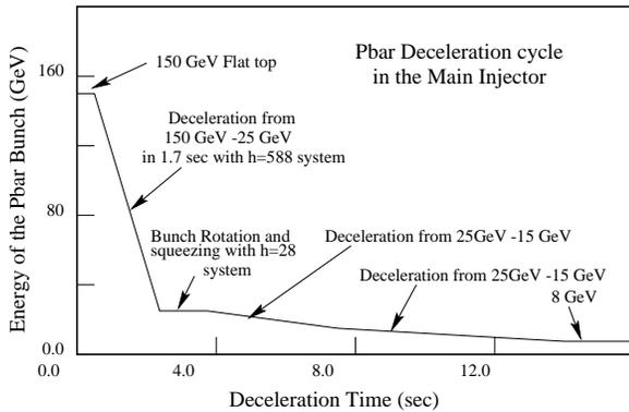
Figure 3: A 12.5 sec long  $\bar{p}$  Deceleration cycle used for simulation.
