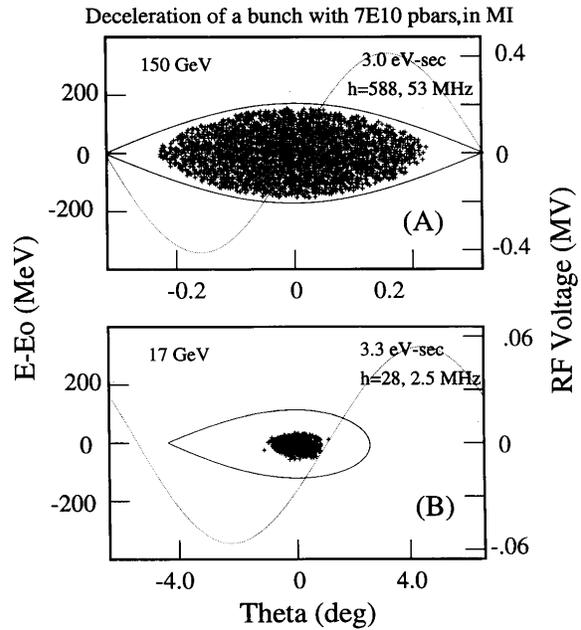
Figure 4: ( $\Delta E$  vs  $\Delta\phi$ ) distribution of the particles in a decelerating bucket of Main Injector. A) 53 MHz rf system at 150 GeV, B) 2.5 MHz rf system at 17 GeV. For other details see caption of Fig. 3.
