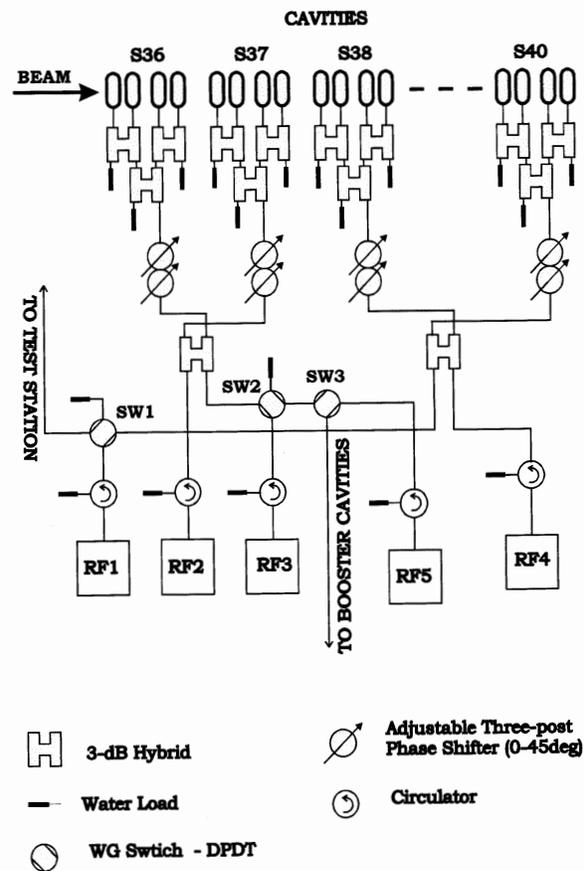
Figure 1: Reconfigurable waveguide switching system.
