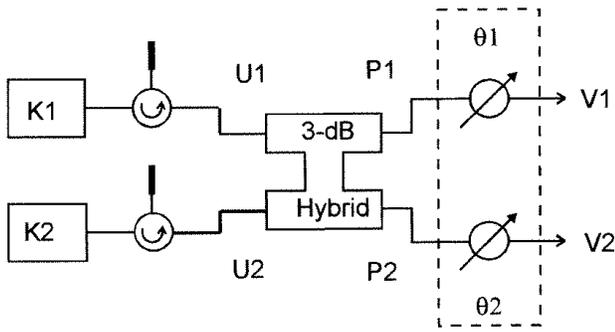
Figure 2: Two klystron-two sector feeding through a hybrid.
