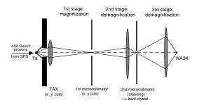
Figure 1: Conceptual layout of the H8 micro-beam (horizontal projection). For the present experiment, the cleaning collimator was removed, the bent crystal installed at its place and the beam tuned to be parallel at the crystal. For details, see text.
