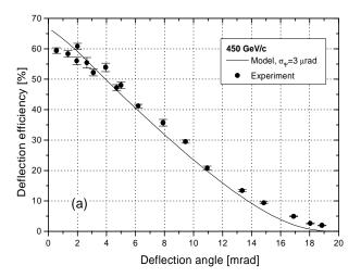
Figure 5: Deflection efficiencies measured for 450 GeV/c protons incident on a bent germanium crystal (dots) compared to calculations following the model of [6]. For details, see text.
