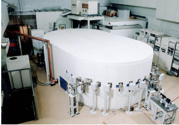
Fig. 5 Photo of A2S after covered with the polyethylene neutron shielding.
