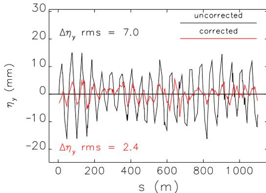
Figure 4: Reduction in  $\eta_y$  by matrix correction
