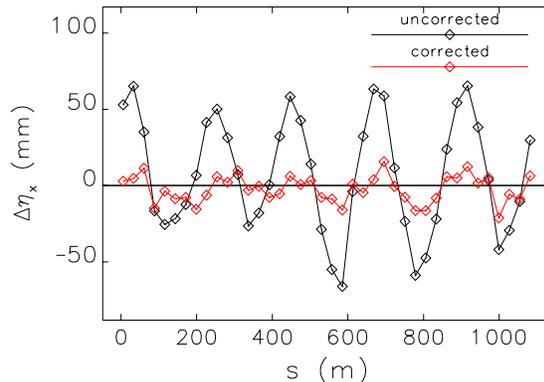
Figure 3: Reduction in  $\eta_x$  error by matrix correction
