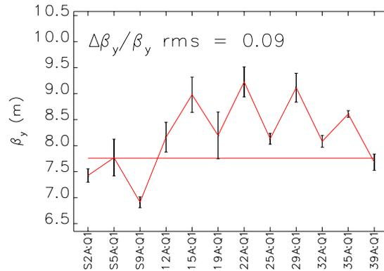
Figure 6:  $\beta_y$  modulation after correction
