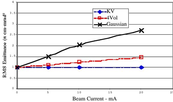
Figure 4. Rms Emittance at EM02 as a function of effective beam current for various assumed beam distribution
