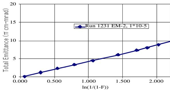
Figure 5. Total Emittance versus fraction of beam enclosed
