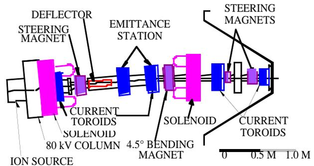
Figure 1 Line Drawing of the Dome LEBT
