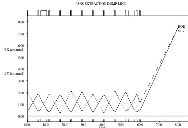
Fig 3. TRANSPORT output showing beam optics to the ring extraction dump.
