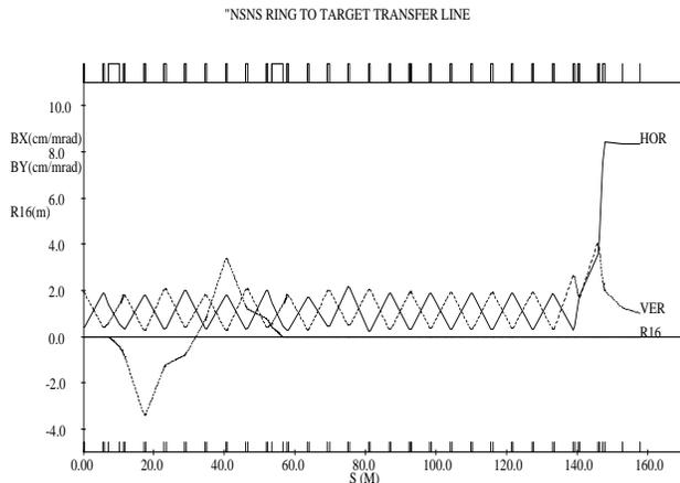
Fig 2. The amplitude function ( $\beta_x, \beta_y$ ) and the dispersion function ( $\eta$ ) along the RTBT.
