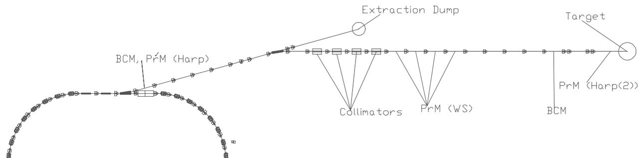
Fig 1. Layout and diagnostics location of the RTBT.
