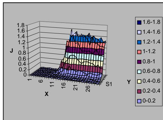
Fig 4. Current density distribution at the target in units of 10 A/m<sup>2</sup>. Only one quadrant of the beam foot print is shown.
