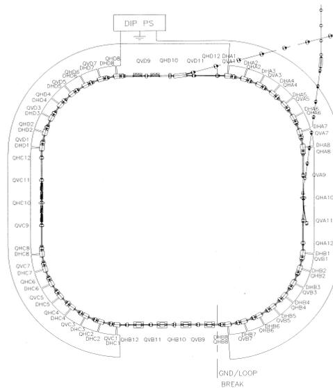
Figure 1: Layout of the SNS accumulator ring.
