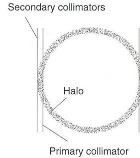
Figure 3: Schematic drawing of the aperture of primary and secondary collimators.
