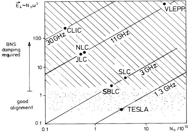
Figure 1: Transverse wakefield  $\vec{E}_\perp$  as a function of bunch population  $N$  for scaled structures with frequencies as considered by the respective linear collider schemes. The hatched area indicates the region where BNS damping techniques will be indispensable, while for the dotted region good alignment of quadrupole lenses and cavities (in the 10 to 500  $\mu\text{m}$  range) may be sufficient.
