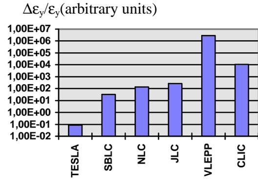
Figure 2: Relative vertical emittance growth (in arbitrary units) from transverse wakefields if cavities are misaligned by  $\Delta y_{\text{cav}}$  and if no BNS damping is applied.
