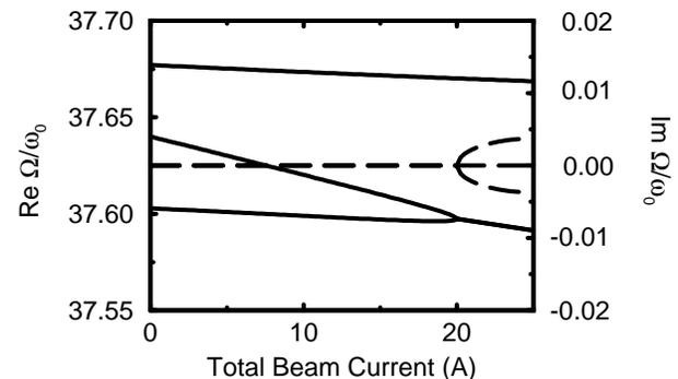
Figure 1. Single bunch mode coupling. Solid lines are real part, dashed lines are imaginary part.
