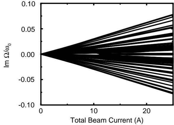
Figure 5. Multibunch  $m = 0$  growth rates, with coupling.
