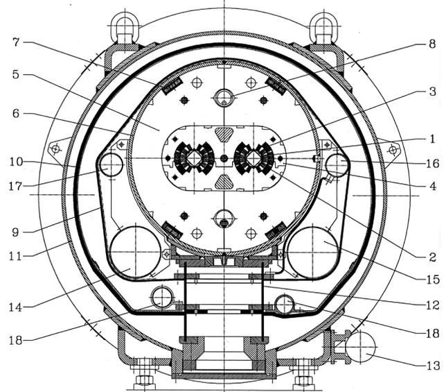
Figure 3: Cross-section of LHC dipole in its cryostat.
