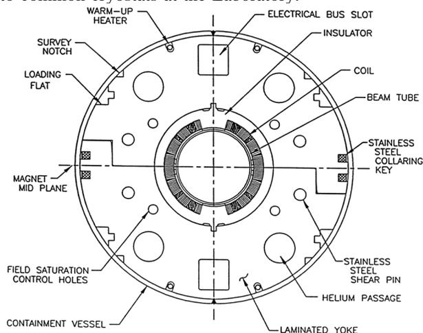
Figure 1: Cross-section of RHIC dipole cold mass.
