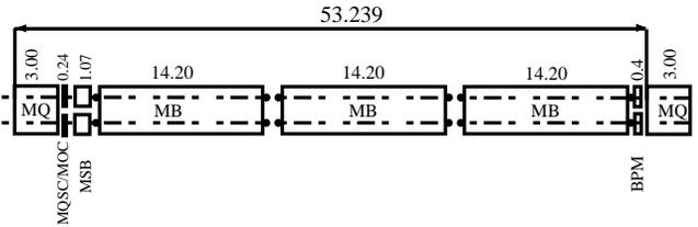
Figure 2: Schematic layout of the LHC half-cell.
