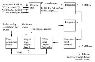
Figure 5: MPS BCM implementation block diagram.
