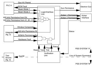
Figure 4: PSS BCM implementation block diagram.
