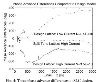
The measurement shows: About 360° change over the length of the linac for FFTB, two big changes in Sector transition 200 m and 400 m where the quadrupole spacing changes by a factor of two for high current design lattice case, and some positive phase for the split tune case.
