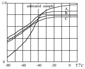
Fig.2. The silicone rubber (mark 9Ì4218, Caterpillar Inc.) module of elasticity  $Å(O)/Å_1$  relative change vs. temperature O for various values of an absorbed doze of electron beam irradiation (absorbed doze increases from sample A to sample C)
