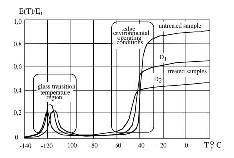
Fig. 1. The silicone rubber module of elasticity relative change E(T)/To vs. temperature T for various values of an absorbed doze (D1 < D2).
