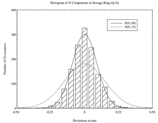
Fig. 6 Histogram of the transverse displacements of all storage ring multipoles
