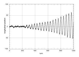
Figure 3. The observed oscillation just after the feedback was turned off. The horizontal axis is the turn number and the vertical axis is the longitudinal position in an arbitrary unit.
