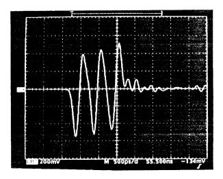
Figure 1. An oscilloscope photo of the pulse train.
