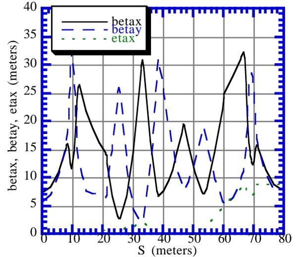
Figure 2: Accumulator lattice -- 1/6th of ring
