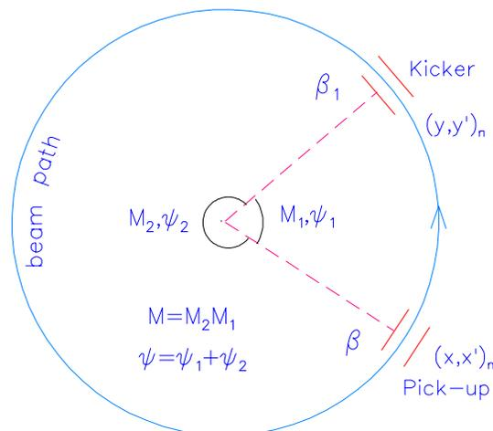
Figure 1. Schematic of a damping system.
