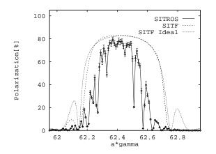
Figure. 5. HERA electron ring with improved dispersion generating vertical bump with optimized spin harmonic content, no beam-beam effect.
