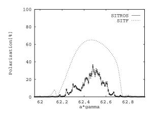
Figure. 2. HERA electron ring with realistically modeled imperfections at the beam-beam limit ( $\xi_z$ =0.04).
