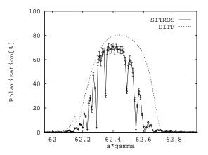
Figure. 3. HERA electron ring without imperfections but with dispersion generating vertical bump. No beam-beam effect.
