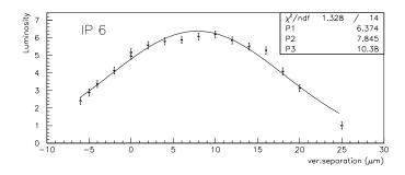
Figure. 3. A complete vertical separator scan around IP number 6. The luminosity is displayed as a function of the vertical separator trim. A Gaussian distribution has been fitted to the data points. The optimum separator settings corresponds to 7.9  $\mu$ m. The width of the distribution is 10.4  $\mu$ m
