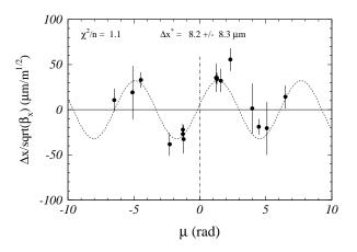
Figure. 4. Example of a fit of the horizontal  $e^+e^-$  difference orbit after adjustment of the horizontal trim separators. The horizontal difference orbit, normalized by the square root of the horizontal betatron function  $\beta_x$ , is shown as a function of the phase advance  $\mu$  with respect to the IP. The fitted horizontal offset  $\Delta x^*$ at the IP is  $8.2 \pm 8.3 \,\mu$ m.
