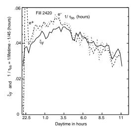
Figure. 2. Evolution of the vertical beam-beam tune shift  $\xi_y$  in the same coast that is shown in figure 1. After a short time  $\xi_y$  settles down above 0.04. The beam lifetimes in collision  $\tau_{bb}$  are correlated to  $\xi_y$  because they are limited by the beam-beam Bremsstrahlung, particularly at lower beam currents. The single beam lifetime of 45 hours has been subtracted from the lifetimes shown in the figure.
