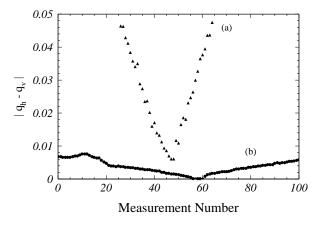
Figure. 6. Difference between the horizontal and vertical tunes for two closest tune approach measurements. Curve (a), where the coupling compensation is poor, corresponds to the measurement shown in figure 5. The lower curve (b) shows a measurement for a machine with low residual coupling between the two planes.
