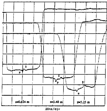
Fig. 10. Current profiles along channel with initial perturbation propagating as fast and slow waves.
