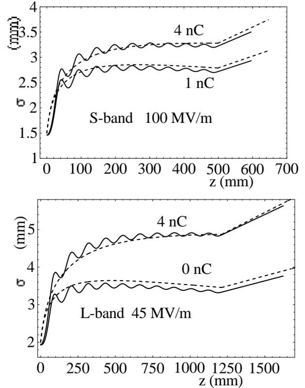
Figure 1: Beam envelopes through two different 10+1/2 cell RF guns ( $\nu=2.856$  GHz upper diagram,  $\nu=1.3$  GHz lower diagram). Dashed lines give the secular orbits analytically predicted, while solid lines are numerical simulation results.
