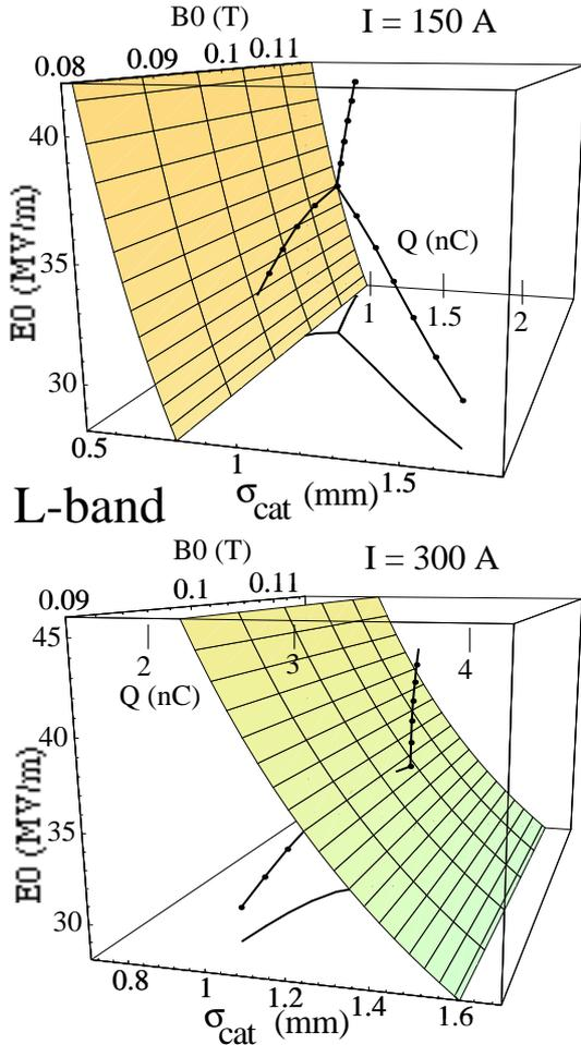
Figure 3: Solutions of eq.7 at  $v=1.3$  GHz,  $A=1$ ,  $I=150$  (upper diagram) and  $I=300$  A (lower diagram), represented by the solid-dotted lines in 3-D sub-space  $(E_0, B_0, \sigma_{cat})$ . Since the bunch aspect ratio is kept constant, the displayed bunch charges are given by  $Q = \sqrt{2\pi} I \cdot \sigma_{cat} / A$ .
