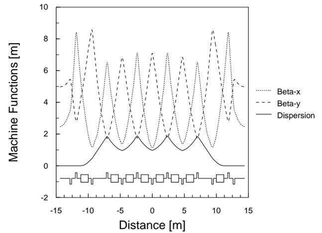
Figure 2. Beta functions and dispersion function for the storage ring under designing.
