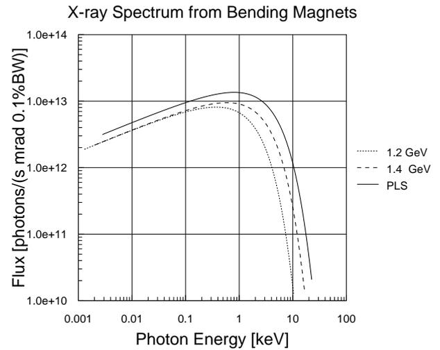
Figure 3. Photon flux per unit horizontal angle as a function of photon energy. The beam current is assumed to be 300 mA. dotted lines are for the storage ring under designing and solid line is for PLS.
