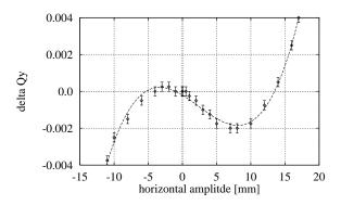
Figure 3. Measured tune shift with horizontal amplitude in the wiggler ASYH. The multipole coefficients obtained from the fit are  $b_2 = 1.0 \pm 0.25 \text{T/m}$  and  $b_4 = -6000 \pm 1000 \text{T/m}^3$ .
