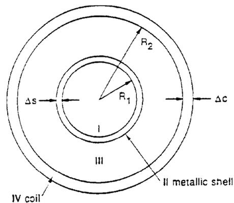
figure 1. Infinitely long metallic shell in solenoidal magnetic field
