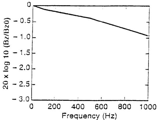
figure 5. Magnitude of magnetic frequency response
