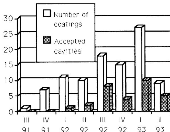
Fig. 3 - Production and acceptance rate of NbCu cavities
