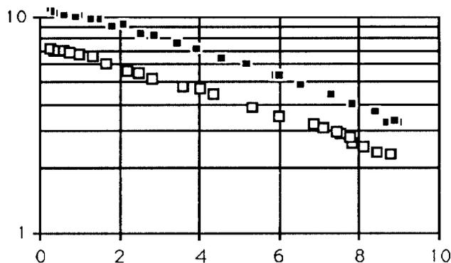
Fig. 2 - NbCu accepted cavities, best and worst :  $Q_0$  vs  $E_{acc}$
