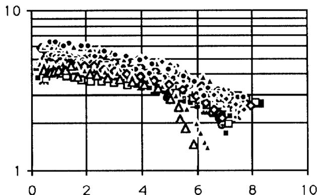
Fig. 1 - Bulk Nb cavities:  $Q_0$ [E9] vs  $E_{acc}$  [MV/m]
