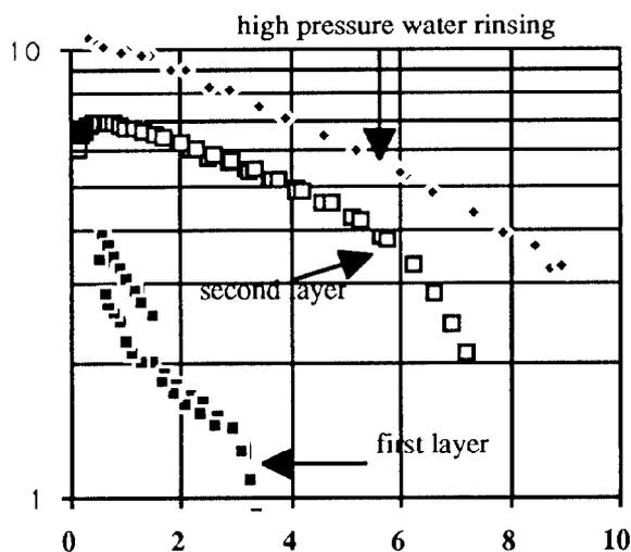
Fig. 3 - Successive coatings:  $Q_0$  vs  $E_{acc}$
